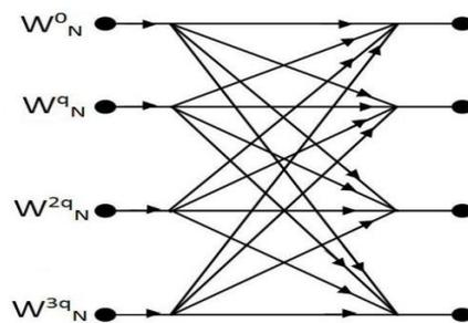
**Fig. 2** Butterfly element for Radix- 4
