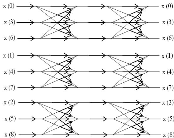
**Fig. 1** 9-point Radix-3 DIT Algorithm
