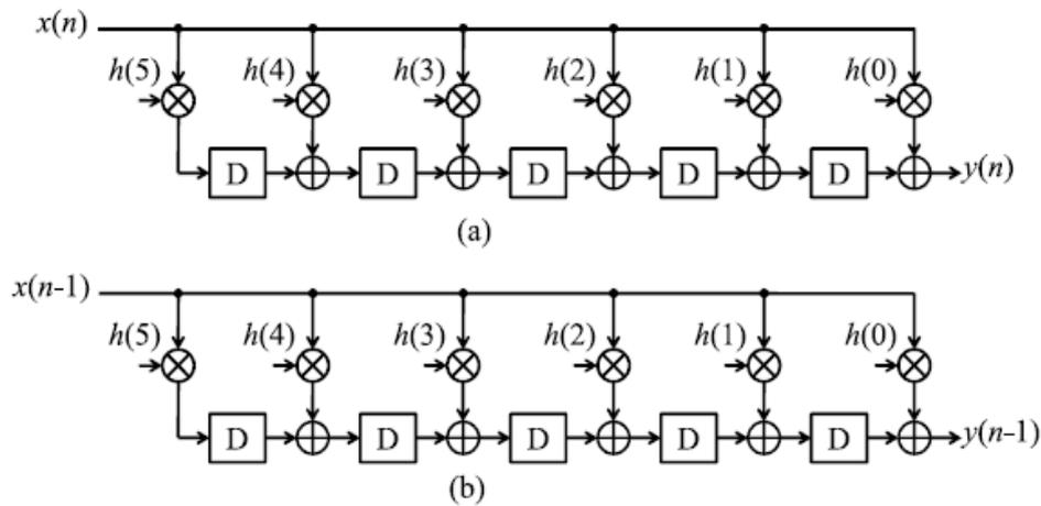
Fig. 1: DFG of transpose form structure for  $N = 6$
