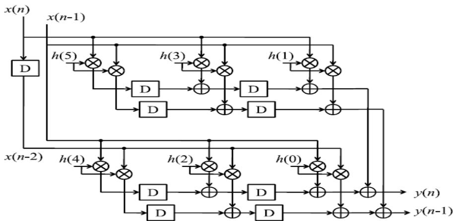
Fig. 2: Merged DFG (DFG-3: transpose form type-I configuration for block FIR structure)
