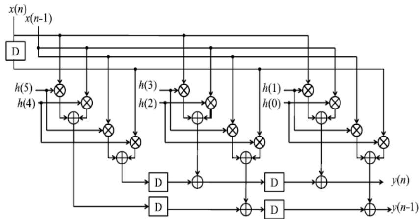
**Fig. 3:** DFG-4 (retimed DFG-3) transpose form type-II configuration for block FIR structure
