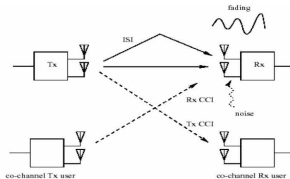
**Fig.2** Fading in MIMO channel.
