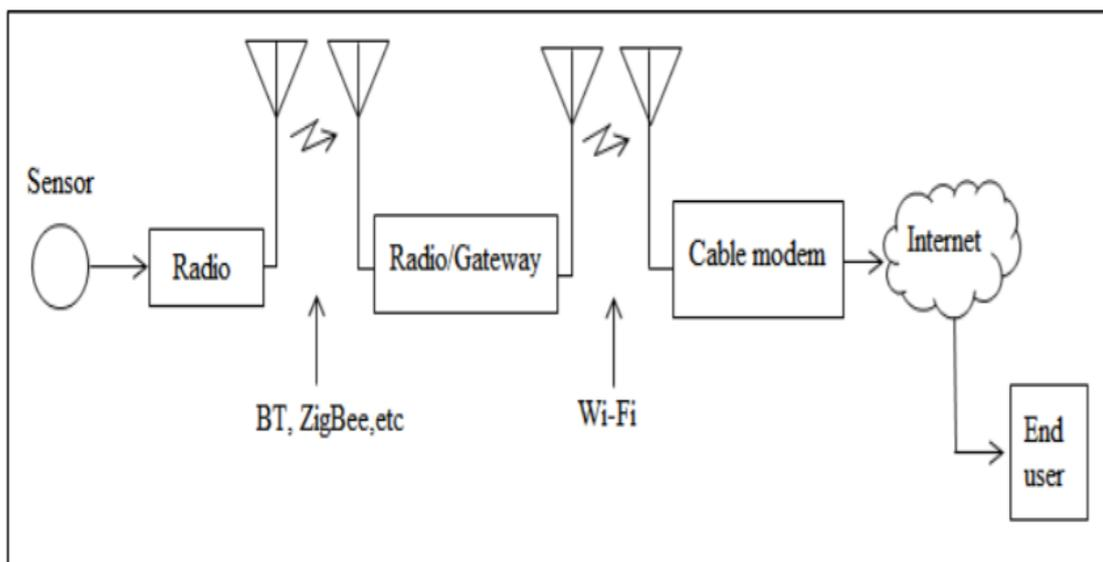
**Fig. 2** Wireless-connection scenarios for IoT
