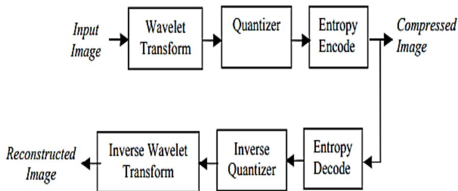
**Fig. 2:** The structure of the wavelet transform based compression.
