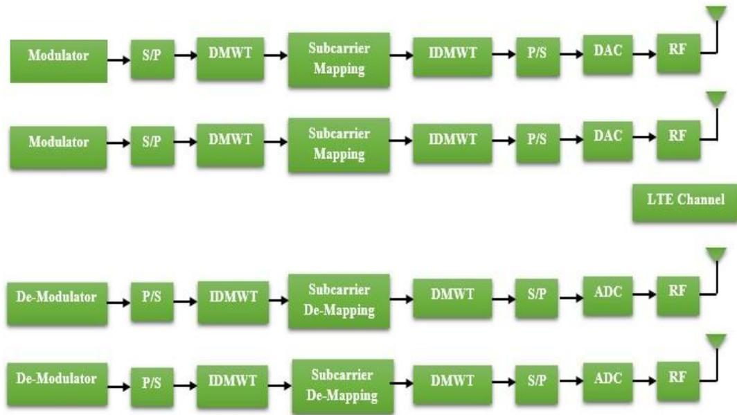
**Fig. 2** Proposed SC-FDMA-DMWT Based Wireless Communication Networks
