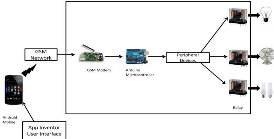
**Fig. 3** Layout of a GSM-based home automation system [23]
