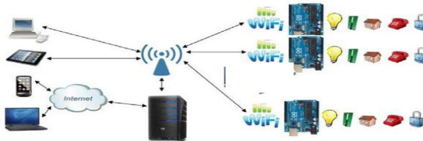
**Fig. 2** A proposed home automation system layout [17]
