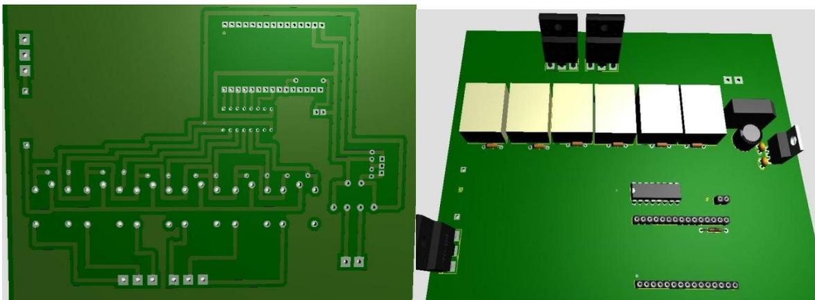
**Fig. 5** PCB designs of hardware and complete circuit diagram of hardware
