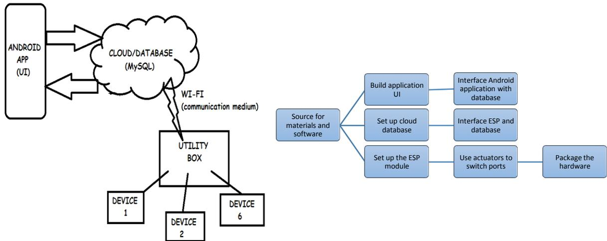
**Fig. 4** Flow diagram and the critical path diagram of the system
